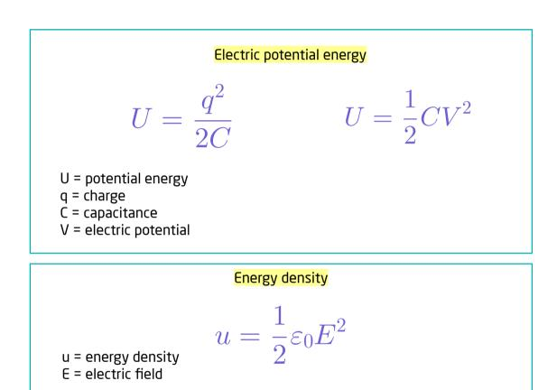
Q12. An capacitor has a charge of 3 nC and applied by electric potential of 12 V, find the potential energy stored in the capacitor
