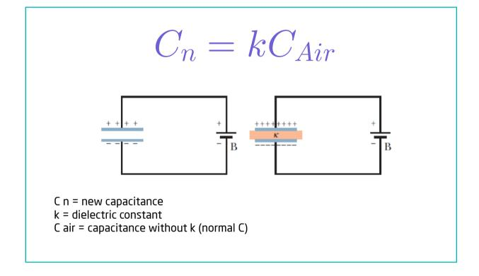
Q13. A capacitor plates with capacitance of 15 nF is charged by a battery to a potential difference V = 12.5 V a dielectric material is slipped between the plate to make the capacitance = 97.5 nF. Find the dielectric constant (k).
