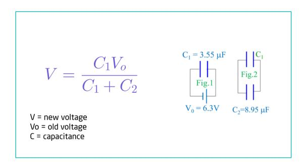
Q9. Example: The battery in fig.1 is removed and replaced by uncharged capacitor  $C_2$  as shown in fig.2. Find the charge on each capacitor in fig.2
